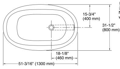
如果与所示的排水管 连接 测量值没有变化(18355T) No change in measurement if connected with drain illustrated.(18355T)
